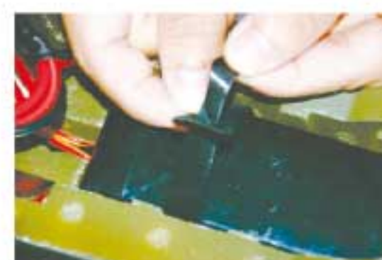
19. Tie up the Velcro to secure the battery.
