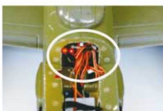
17. Chamber for the wires.
