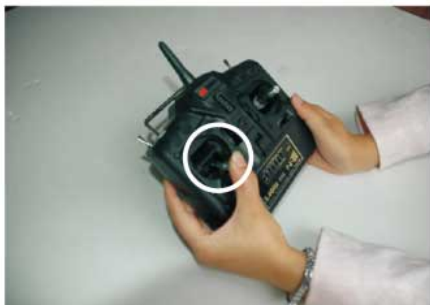
1. Throttle in lowest level, the same with trim.
