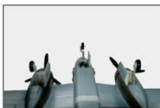
24. Switch the Ch5 several times to adjust the landing gear. Note: Keep the throttle and trim in the lowest position before operating on the CH5.
