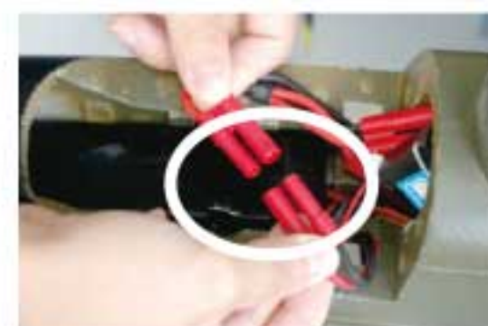
22. Connect the battery.
