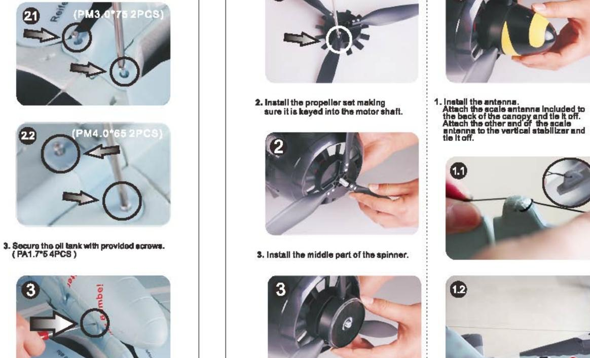
installing the propeller and small parts
