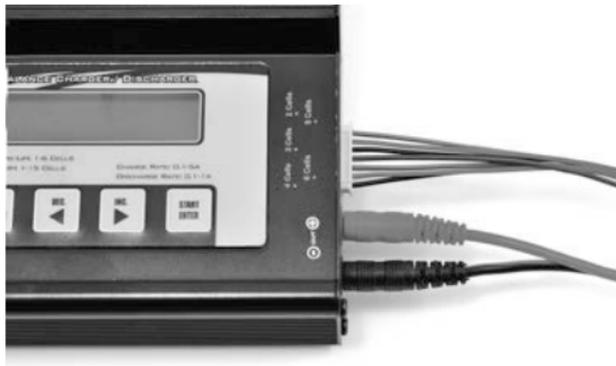
The main battery leads must be connected along with the balance lead connector as shown before charging your battery.
