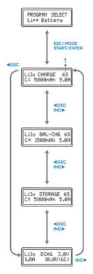
Once you power on the charger, press the MODE/ ESC key. This will shift you down to the "Program Select" menus. Navigate with the ESC/MODE and <DEC keys until you reach your desired Lithium battery type; be sure to select the correct battery type! Then press the ENTER/START key to store the value. Press the ENTER/START for more than 2 seconds to start the process.
