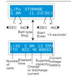
At this screen, you can set up the current and voltage of the battery pack. Charging and discharging will make the batteries come to the voltage level of 'storage' state.
