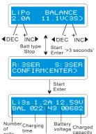
The left side of the first line shows the type of battery you choose. The value on the left of the second line of the charger is current user set. After setting the current and voltage, press START/ENTER key for more than 3 seconds to start the process. (charge current: .1-5.0A, voltage: 1-5V).
