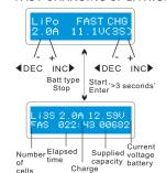
Charging current will decrease as it reaches the end of charging. A specific CV process will be reduced to end the charging process earlier. In fact, the charging current will goes to 1/5 when the charging process comes to 1/10. Charging capacity will be a little smaller than normal charging, but charging time will be shortened accordingly.
