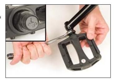
Note: You will damage the threads in the crank arms if you thread the wrong pedal into the wrong crank arm.
