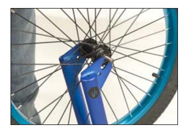
Note: Some front hubs require the fork legs to be spread apart a little for the axle hardware to clear the inside of the dropouts. This will not damage your forks!
